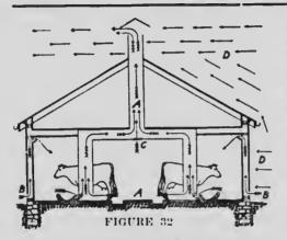
Section of dairy stable showing the action of the wind at D D, forcing air into the stable by direct pressure at B B and out of it by suction at the top of the ventilating shaft A. At C is a ceiling register in the ventilating shaft, to be opened only when the stable is too warm or when the draft is too feeble. (From "Veatilation for ibwellings, itural Schools and Stables", by F. il. King.)
