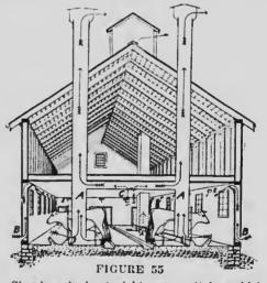
Showing single straight-away outtakes which avoid all angles and render possible the strongest draft. A A are the two outtakes; B B are the intakes; C, a celling register in the cross-arm joining the two sides of the outtake. (From "Ventilation for Dwellings, Rural Schools and Stables", by F. II. King.)
