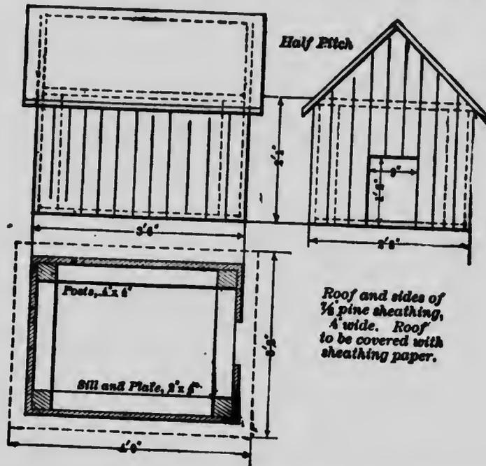
sheathing-boards on each side? How many on each end? How many square feet of sheathing-boards, allowing 20% waste? What will the sheathing-paper for the roof cost at 4¢ a square yard?
