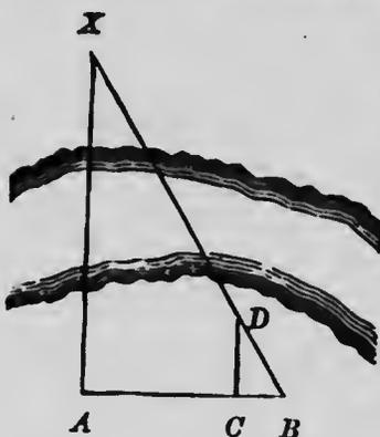
5. To find the distance from  $A$  to the inaccessible point  $X$ : Draw  $AB$  perpendicular to  $AX$ . Join  $BX$ . Draw  $CD$  parallel to  $AX$ . What kind of angles at  $A$  and  $C$ ? What two similar triangles? What sides are measured? What is the proportion? Show how you can find the distance from  $B$  to  $X$ .
