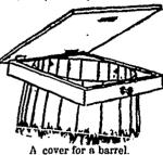
easily-closing lid. The engray. ing represents a famous sort of cover, to which an ordinary lock can be easily fitted. A frame is applied to the outside of the barrel, which fixes itself on the sides, to which it is fastened by screw bolts. Hinges attach a flat-lid to the frame, and the lock can be easily added.
