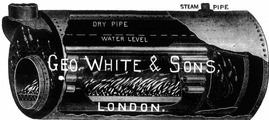
This style of boiler is used with all our threshing engines, enabling our customers to produce abundant steam with long, rough, cheap wood. We utilize water space surrounding and at back end of fire box in connection with our improved internal straw burner.
