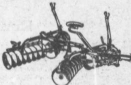
The frame on the Bissell Harrow is directly over the gangs, the draught being well back while the work is being done. The horses do not have to carry the weight of the pole, levers, braces or frame. This feature is important, and herein lies one great advantage of Bissell Disk Harrows.
