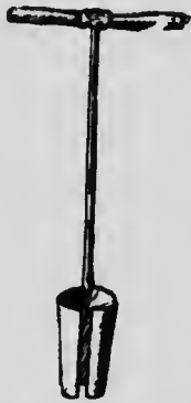
Fig. 3.—Hollow spade for transplanting coniferous seedlings.
