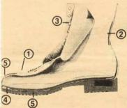
CSA approval as a safety boot means approval of materials and construction.
