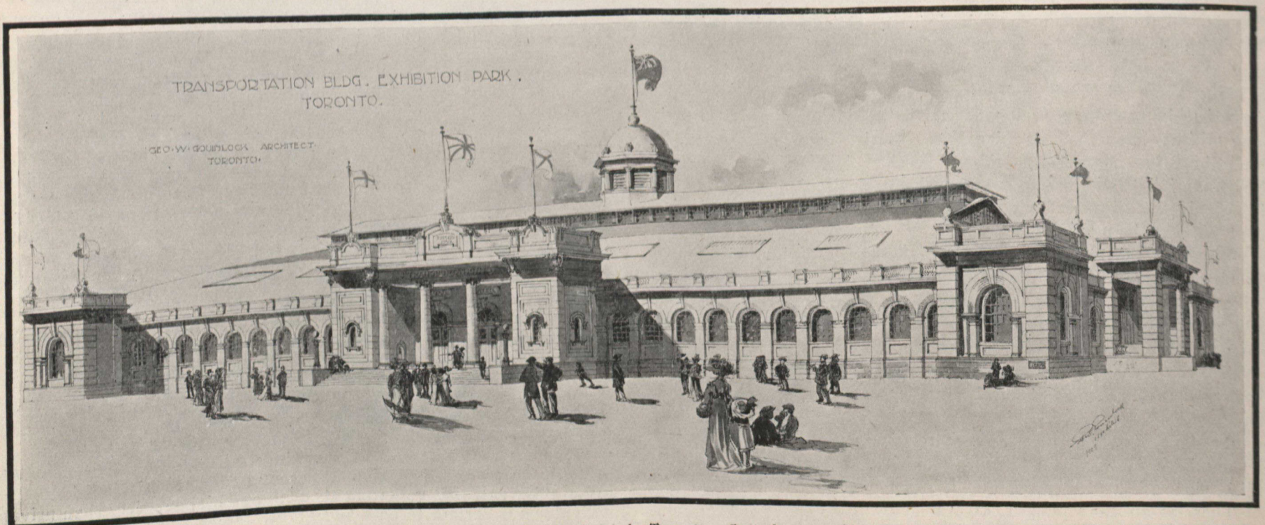
A New "Transportation" Building now being erected on the Exhibition Grounds, Toronto. Cost, $95,000. Size, 337 feet by 153 feet. Materials, Steel, Red Brick and Stone Trimmings. Architect, Mr. George W. Gouinlock. Corner Stone Laid last Monday.
