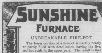
the upper portion expands much more than the This uneven expansion causes a strain too great for a one-piece fire-pot to stand. Sooner or later it will split, allowing precious heat and sickening gases to But the fire-pot of the Sunshine is constructed to meet this condition. It is in two sections. The upper half expands, as much as
