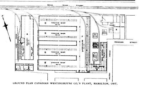
of the foundry and warehouse, along with corresponding machine shop wings, being left for future extensions. Regarding progress of material through the plant, it may be pointed out that with raw material received on track west of the foundry, progress is in general from this point to the warehouse, from which all shipments are to be made over tracks conveniently located within the building for this purpose.
