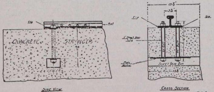
**Fig. 3.—Details for Concrete Stringers, Showing Old Method of Fastening Rails.**
