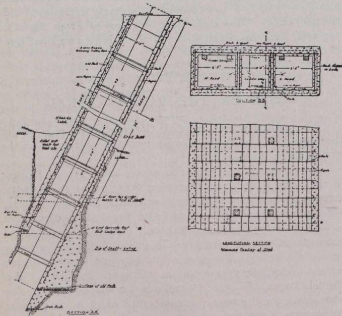
**Fig. 2.—Reinforced Concrete Collar, No. 3 Shaft, Trimountain Mine.**
