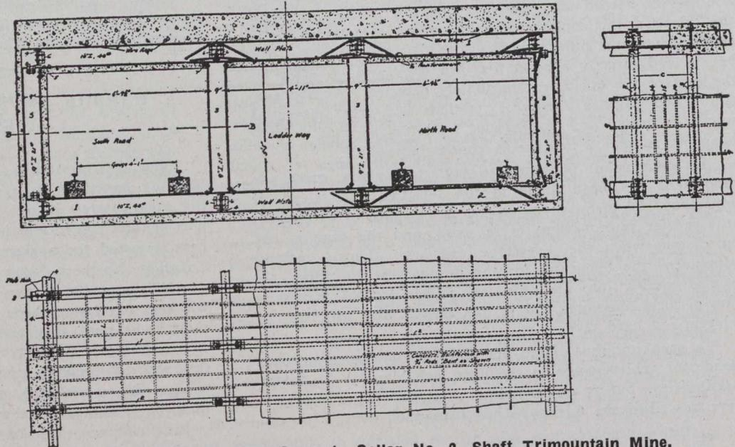
**Fig. 1.—Details for Steel-Concrete Collar No. 2. Shaft Trimountain Mine, Plan and Elevation.**
