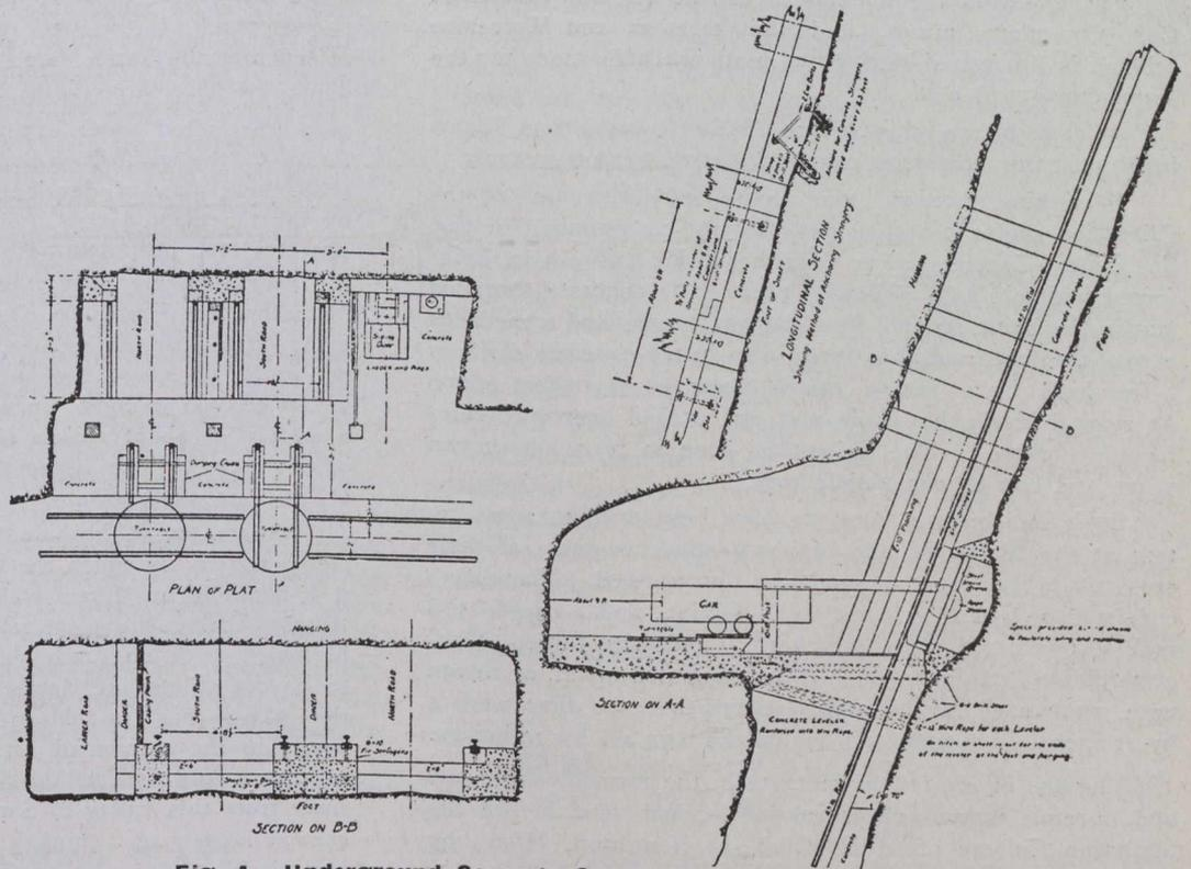
Fig. 4.—Underground Concrete Construction, Champion Mine.
