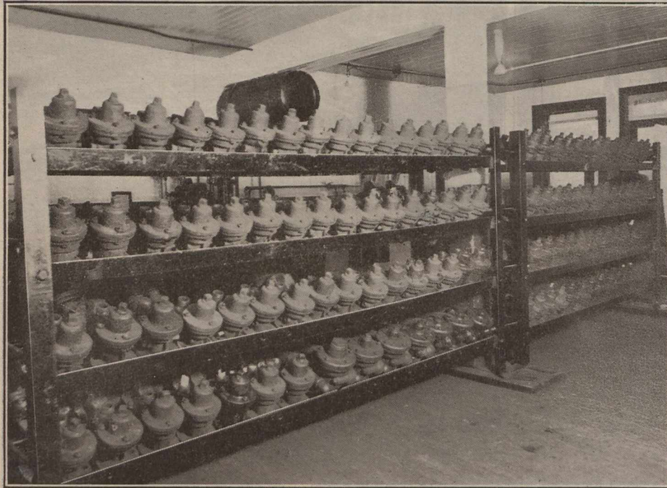
Racks for Holding Triple Valves.
