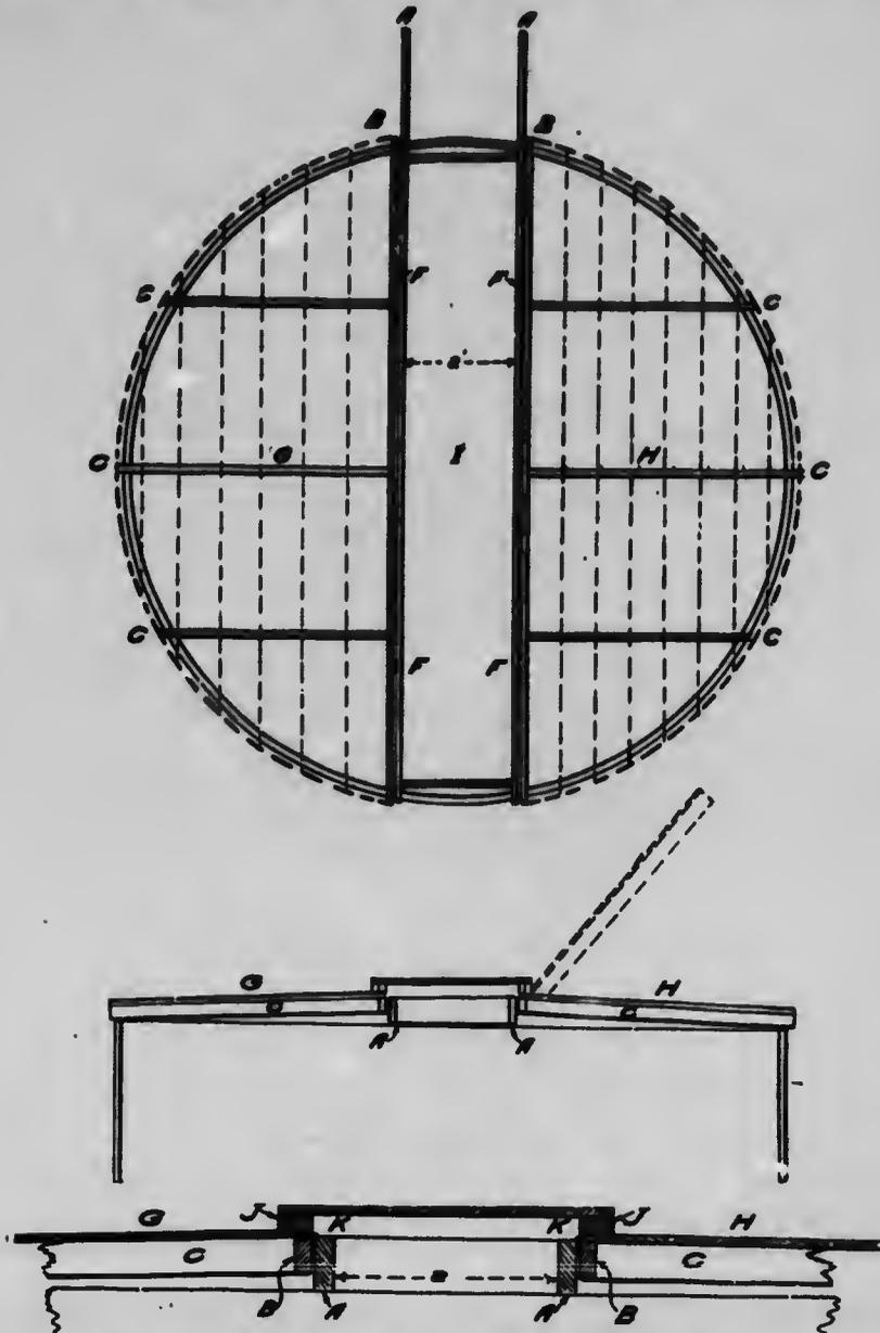
Fig. 11. Diagram of silo roof. A, 2" x 6"; B and C, 2" x 4"; F, hinges; J and K, 2" x 4". The roof is in three sections, G, H, and I. G and H are hinged to the frame A-A, and may be tipped up when the silo is nearly full to allow filling to the top. The sliding door, I, can be moved to either side and leaves an opening for the blower to deliver into.
