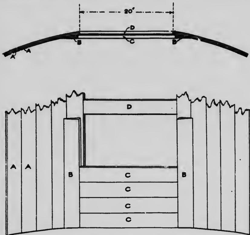
Fig. 10. Diagram of silo door. A. Silo wall, 2" x 6" staves. B. Door-jamba, 2" x 6", diagonally cut. C. Sections of tongued and grooved staves filling the continuous opening. D. Braces keeping the staves apart to form the continuous opening.
