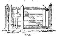
holds the top of the lever to the gate. E, figs. 1 and 2, is the wire in position, A,A, are the pieces or bolts that go into the mortices in the posts; they are fastened to the upright E, and this is attached to the lever D, by the connecting piece C. It should be fastened by a bolt at each end, loose
