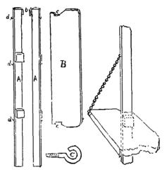
The shelves, B, are eight inches wide, with notches, cc, cut at each end to accommodate the uprights. The distances between these notches should be just two inches less than the width of the window, so that the whole may fit closely when in place. The form is that of an upper shelf, the dotted lines representing those which rest against the lower sash. At each end of the shelf is a screweye, ff, with a chain one foot long attached.
