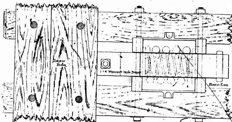
This illustration represents a set of No. 68 Butler Drawbar Attachments, applied as we recommend. We show an  $1 \times 4$  inch wrought strap or yoke, a less size can be used if desired. Yoke cannot get out of place on account of side walls. No bolt through center necessary to hold springs in position.
