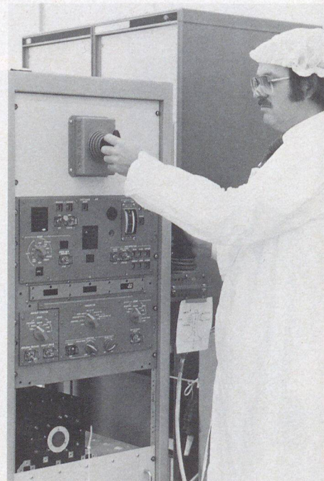
Hand control systems for CANADARM were developed by CAE in Montreal.
