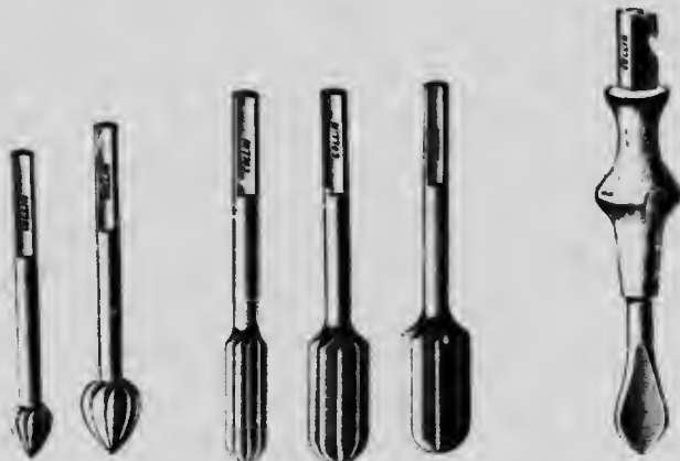
FIG. 401. — FLAT POINTED DRILL OF 12 MILLIMETRES DIAMETER, MOUNTED ON THE HOLDER OF A TREPAN À CLIQUET.
