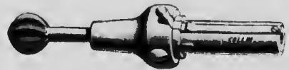
FIG. 398. — SPHERICAL BURR OF 12 MILLIMETRES DIAMETER, MOUNTED ON A HANDLE ADAPTED TO ELECTRIC INSTRUMENTATION.
