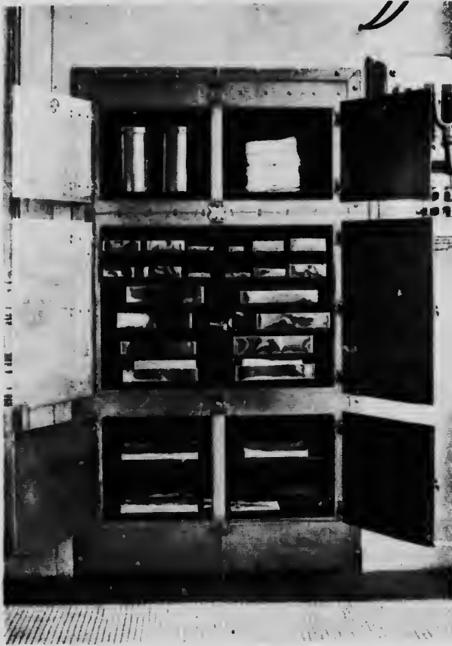
FIG. 22.—AUTHOR'S DRY-STOVE FOR STERILIZATION: THE LARGE MODEL.
