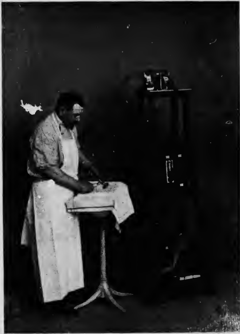
FIG. 399. ELECTRIC MOTOR, FLEXIBLE TRANSMITTING CABLE, HANDLE WITH VARIABLE INCLINATION, AND CIRCULAR SAW.
