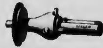
FIG. 395.—SAW OF 35 MILLIMETRES DIAMETER, MOUNTED, AND FURNISHED WITH A PROJECTING RIM WHICH LIMITS THE DEPTH OF THE SECTION.
