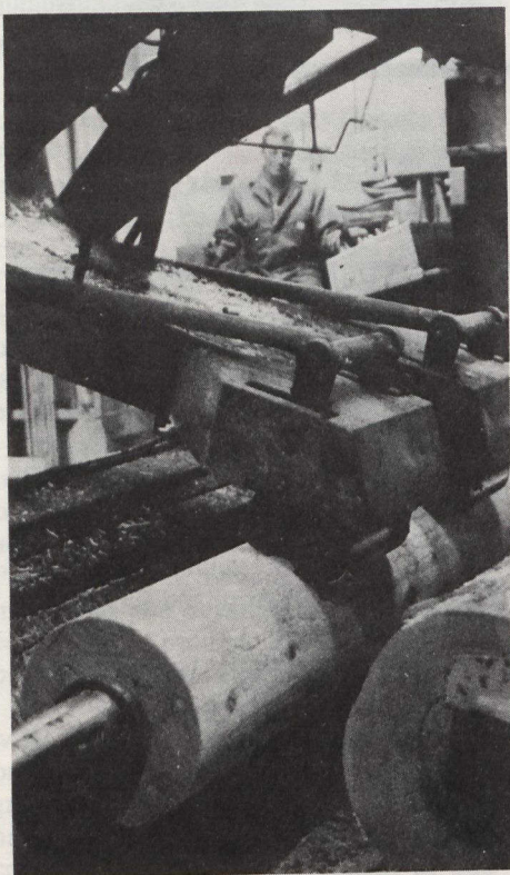
Huge lathe peels a Douglas fir log into sheets of veneer for Canfor plywood. The Canfor Group of companies – Canadian Forest Products Ltd. and its affiliates – is based in Vancouver, British Columbia.
