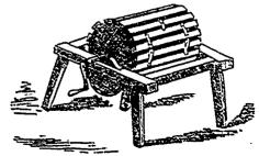
inch plank, and the slats one inch thick, two inches wide and three-fourths of an inch apart. The door is put on with a pair of strap hinges as represented. Roots may be completely washed by revolving the lower part of the machine in water.
