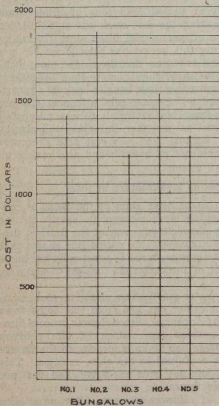
FIG. 1—VARIATION OF COST OF BUNGALOWS BUILT TO SAME PLAN
