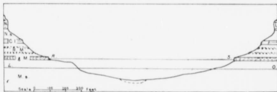
Fig. 17. Section across gorge at Whirlpool, between Thompson point and Colt ravine. Broken line shows river bottom outside this line.
