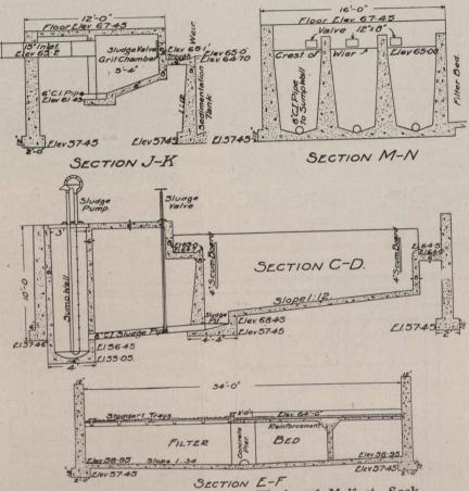
Fig. 6.-Details of Disposal Works of Melfort, Sask.
