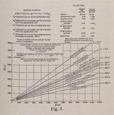
The writer realizes that such a diagram cannot be relied on entirely in the location of a conduit, for there are local conditions on every piece of work which must be taken into account.
