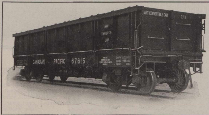
HART CONVERTIBLE CARS Steel or Wood Construction, 30 to 50 Tons Capacity
