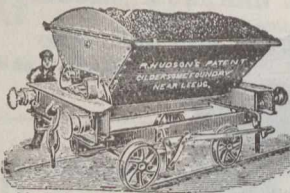
59-R. H.'s Patent 6-Ton Steel Double Side Tip Wagon, to work with ordinary Rly Wagons
