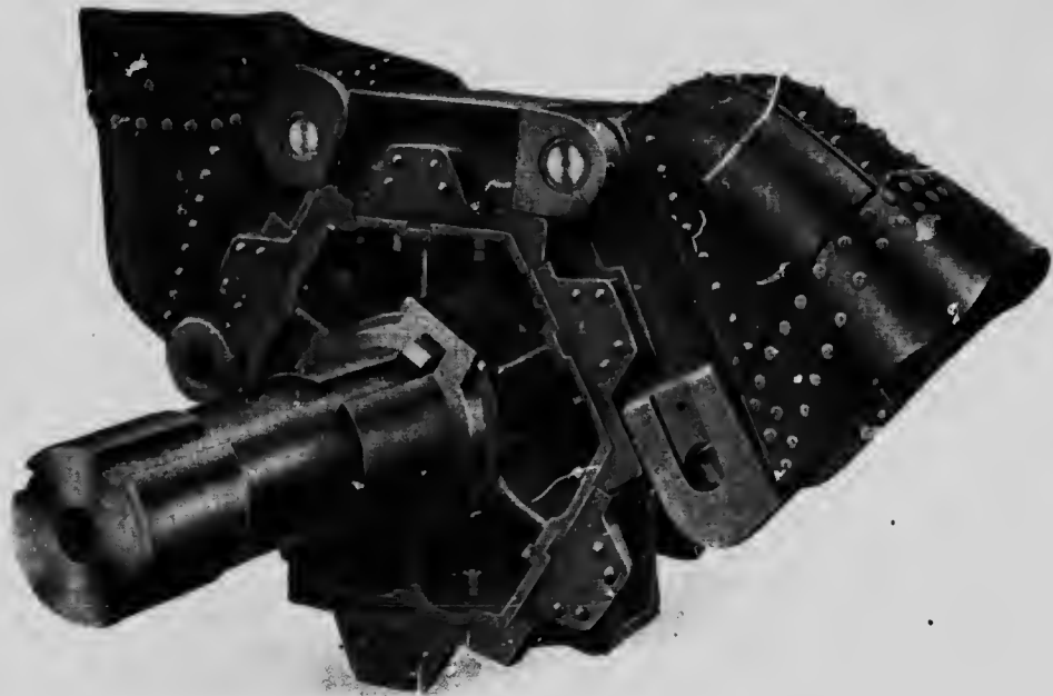
Five and a half Open Connected Buckets and Upper Turbine
