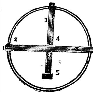
take a strip to reach across the barrel to fit in notches; make round each end so it will turn easily; then take a second piece to go across the barrel flat; allow one end to rest on the edge of the barrel; tack in middle of the first strip, bait by tacking a meat skin on this short end; fill barrel with water, and often one-half bushel rats can be caught in a single night.
