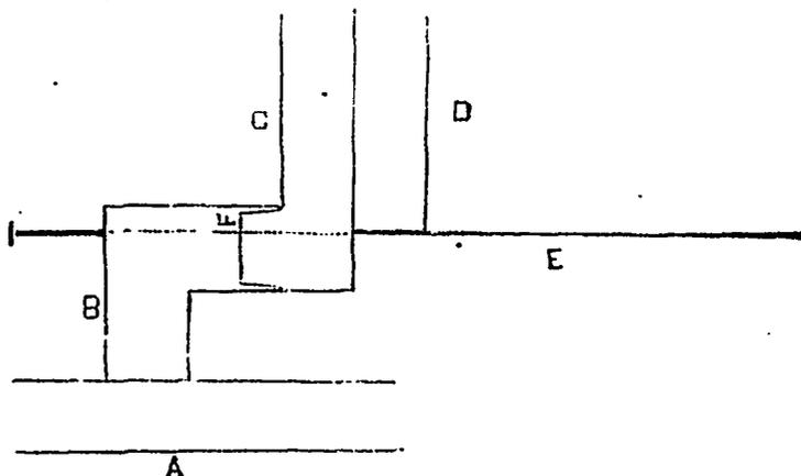
Stovepipe A and elbow B—fixtures. Box D and elbow C turn on support. On moving box right or left, support turns on pivots, as does C.
