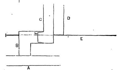
Stovepipe A and elbow B-fixtures. Box D and elbow C turn on support On moving box right or left, support turns on pivots, as does C.
