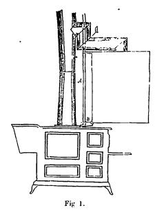
less than in length, that when charged with fruit the draught of the hot air currents may not be hindered. The frames should be steeped in a saturated solution of alum, which will render them incombustible. As the top of the evaporator is about three feet from the stove, it may be made of wood. As to the lower part, the back and sides are fixed on a frame of iron,  $\frac{3}{4}$  of an inch broad, by means of rivets.
