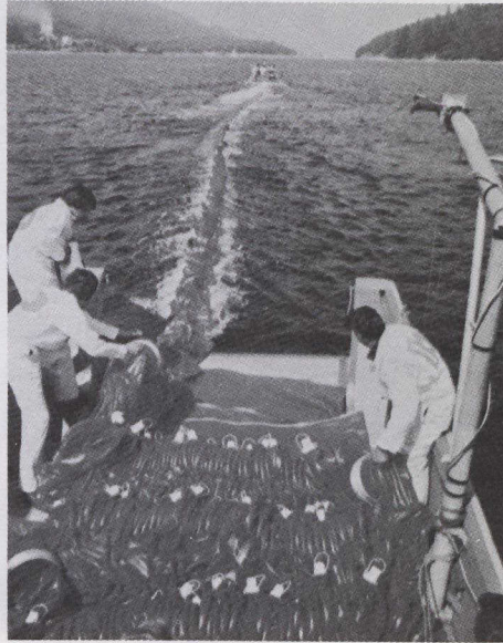
The ZOOM boom is packed in compact casing that releases miles of fencing to trap and contain an oil spill. Disc oil skimmers recover the oil before it can do any harm.
