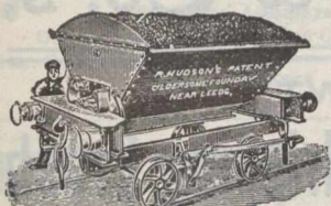
59—R. H.'s Patent 6-Ton Steel Double Side Tip Wagon, to work with ordinary 14 1/2 Wagons
