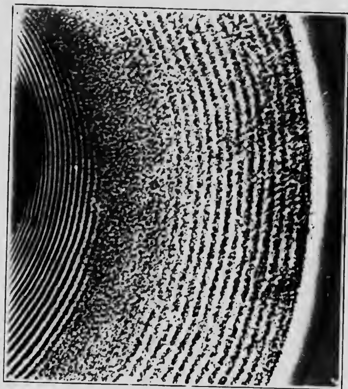
FIG. 2. \times 5 A portion of the same (fig. 1) enlarged to show the character of the precipitate in the "granular" zones.
