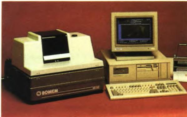
*Bomen offers a complete range of infra-red spectrometers capable of characterizing organic or mineral samples.*
