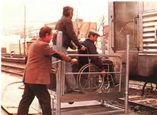
*The wheelchair lift produced by Adaptive Engineering Ltd. is designed for use with rail cars, buses, aircraft, ferries or any situation where a portable device is required for wheelchair access.*
