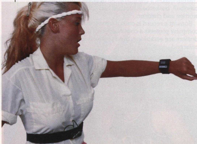
TELE•PULSE™ heart-rate monitor with wrist watch receiver allows interference-free heart-rate monitoring while on the run.
