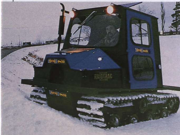
Raidtrac's tractors have a galvanized steel body and laminated glass windshield.
