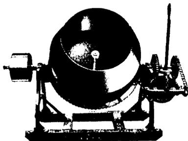
The attention of contractors is particularly called to our Open Drum Batch Mixers. The only Mixer on the market which mixes the material in sight of the operator, permitting proper gauge of the material and moisture desired, and examination as to when batch is ready to dump. It is also cleanable to an extent which entirely eliminates the caking of concrete, imparting to the machine long lasting qualities.
