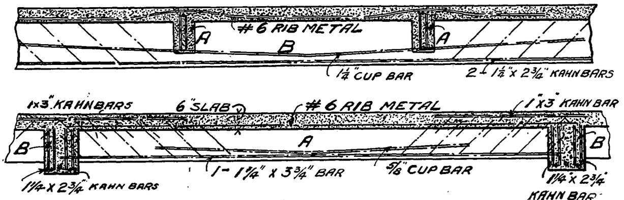
Detail of typical beam and floor construction, Jacobs Building, Montreal. Mitchell and Creighton, Architects.
