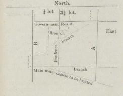
If the preliminary proceedings laid down in The Ditches and Watercourses Act have been taken by A (the party applying for the ditch), and in the opinion of the engineer the proper drainage of A's land requires the three branch drains, then the engineer has authority to make an award providing for their construction, observing, of course, the formalities required by the act.
