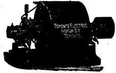
Our new tour-pole Motors, highest efficiency and all latest improvements; built in sizes 10 to 50 h. p. Our Bipolar Motors from ½ to 20 h. p. are not equalled.
