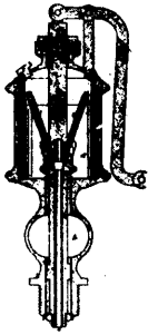
7108 Gowenlock & Mannering's Improvements on Steam Lubricators.
