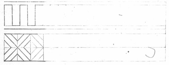
Practice in faint and firm lines. The faint lines are such as should be used for guide, or construction lines, and for the first light sketch of a figure. The darker, or firm lines, are those required for the finished drawing. Draw the lines at equal distances and of the same strength as the examples.
