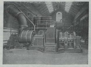
A BELLISS RECIPROCAT-ING ENGINE COMBINED WITH AN EXHAUST TURBINE GIVES UNPAR-ALLELLED ECONOMY.
