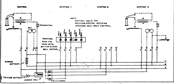
WIRING DIAGRAM SHOWING CONNECTIONS FOR ELEVATOR TELEPHONE.
