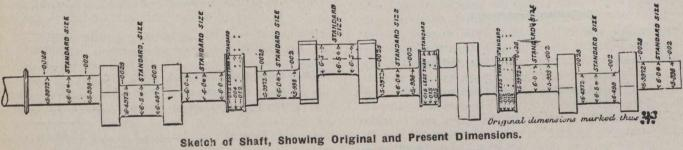
other parts is merely microscopic, it being a noteworthy feature that all the bearings remained cylindrical.
