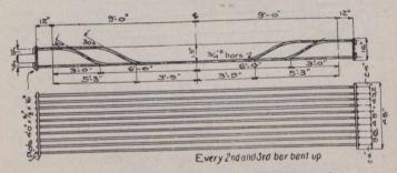
Detail of Shop Built Slab Reinforcement.
