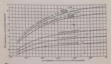
Fig. 3.-Relation Between Wind Pressure and Slope of Roof.
