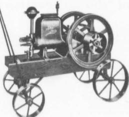
The "STAR-RITE" is a comparatively new engine to the Canadian market, and is put out by the Empire Cream Separator Company of Toronto. It is hopper-cooled, has suction feed for gasoline, and the larger sizes have jump-spark dual ignition—thus always insuring a spark. Simplicity of construction is strongly emphasized in every size, which run from 1/2 H.P. up, and are equipped to perform any work within their power from the churn to the portable sawmill. (See page 51).
