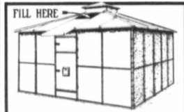
12 ft. x 12 ft. - 6 ft. wall - Capacity 850 Bushels 14 ft. x 14 ft. - 6 ft. wall - Capacity 1100 Bushels
