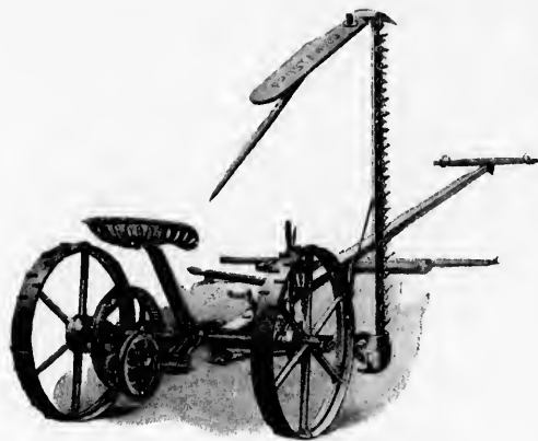
How the Cutter-Bar Folds
