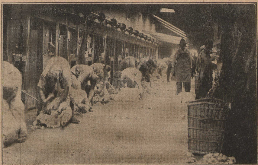
The sheepman's harvest. A view of the shearing board at the Bitter Creek shearing shed, built on the Australian plan. This is a 32 machine plant. Shaft runs overhead, with drop shaft for each shearer. The hum of the machines is now general throughout the south and central western states.
