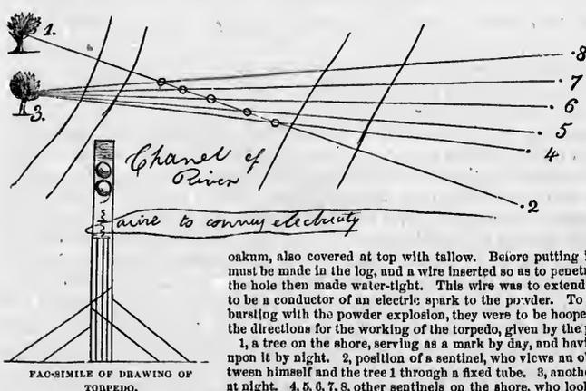
Then fill the place with hot tallow, so that it will thoroughly enter the pores of the wood, and make it impervious to water. Then bore it out again, and put in powder in flannel cartridges. Over the powder place two balls, and then pour in melted tallow again, so as to completely inclose the powder. Over the balls put a wad of
