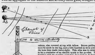
Then fill the place with hot tallow, so that it will thoroughly enter the pores of the wood, and make It impervious to wa-Then bore it out again, and put in powder in flannel cartridges. Over the powder place two balls, and then pour in melted tallow again, so as to completely inclose the powder. Over the balls put a wad of
