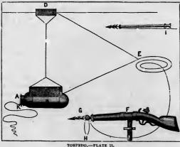
the harpoon parallel to each other, the cope will act like a tail or rod to a rocket, and guide it straight. F is the harpoon gun, acting upon a swivel fixed in the stern-sheets of a boat. The harpoon is fixed in the vessel's
