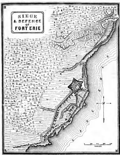
Explanation of the arove Map.—A, old Fort Erie; a, a, demi-bastions; b, a ravelin, and c, c, block-houses. These were all built by the British previous to its capture at the beginning of July. d, d, bastions built by the Americans during the siege; e, e, a redoubt built for the security of the demi-bastions, a, a.
