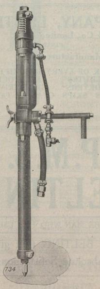
The new CCW-21 Water Stoper has several novel features in connection with the water feed that will at once appeal to the experienced miner.
