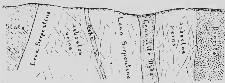
FIG. 3.—Profile of Asbestos-bearing formation at Black Lake and Thetford.
