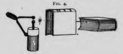
are extremely minute, so that the influence they have in transmitting or obscuring light waves is commensurate with the difference in the oscillation-length of light waves and Hertzian waves. The light which passes through tourmaline, like the electric waves which pass through the leaves of a book held edgewise, have this peculiarity—they oscillate in one plane, and resemble in that respect the waves of the sea. They are said to be polarised.
