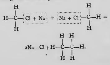
The new gas is called **ethane**. It, too, exists in only one modification, and it is legitimate to suppose that the atoms of hydrogen are symmetrically arranged with reference to the two atoms of carbon.
