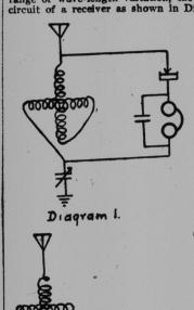
variometer is connected in the same manner as a single slide tuner. When the variometer is adjusted to a low value of inductance, it offers much more resistance to the currents of radio frequency than a tuning coil having the same amount of inductance. For use on the amateur wave length
